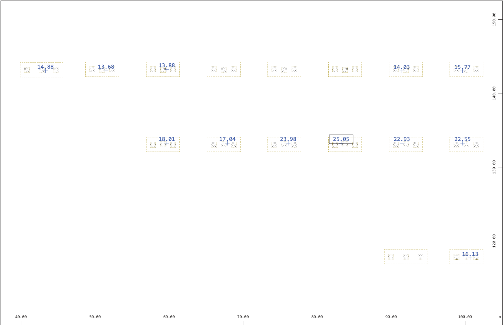
Sector of system Group 2 Quadrilateral Elements , Shear reinforcement in cm2/m2, Design Case 1 , Values greater than 13.26 (Max=25.05)
