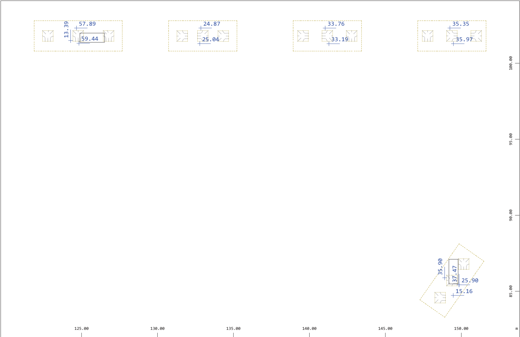
Sector of system Group 44 Quadrilateral Elements , lower Reinforcements in cm2/m, Design Case 1 , Values greater than 13.26/13.26/- (Max=59.44) Y Z-X mispost from Sector 0.005
