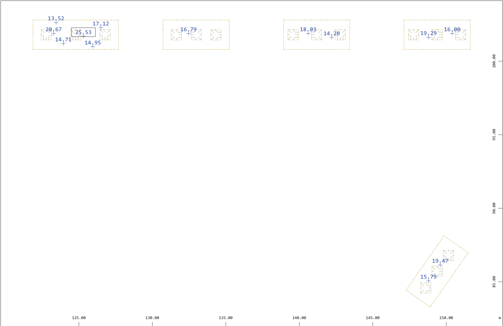
Sector of system Group 44 Quadrilateral Elements , Shear reinforcement in cm2/m2, Design Case 1 , Values greater than 13.26 (Max=25.53) Y Z-X misprint from Sector 0.0015
