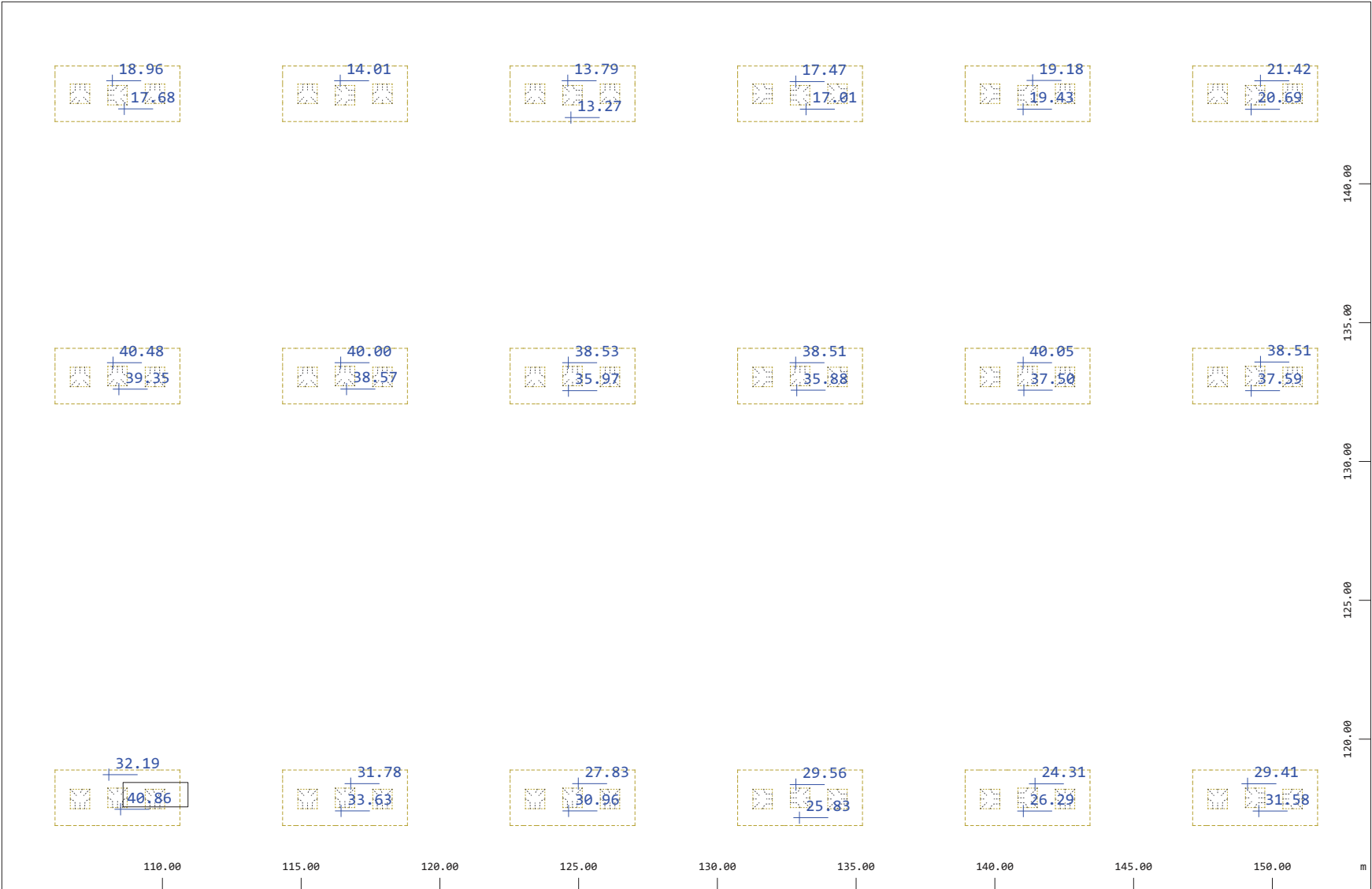
Sector of system Group 15 Quadrilateral Elements , lower Reinforcements in cm 2 /m, Design Case 1 , Values greater than 13.26/13.26/- (Max=40.86) M 1 : 195 Y Z-X 110.00 115.00 120.00 125.00 130.00 135.00 140.00 145.00 150.00 m 120.00 125.00 130.00 135.00 140.00
