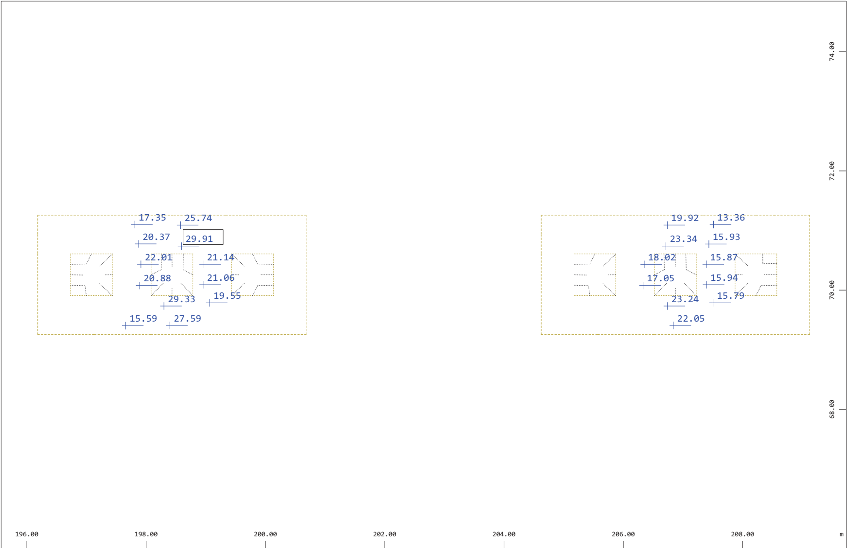
Sector of system Group 70 Quadrilateral Elements , lower Reinforcements in cm 2 /m, Design Case 1 , Values greater than 13.26/13.26/- (Max=29.91)
