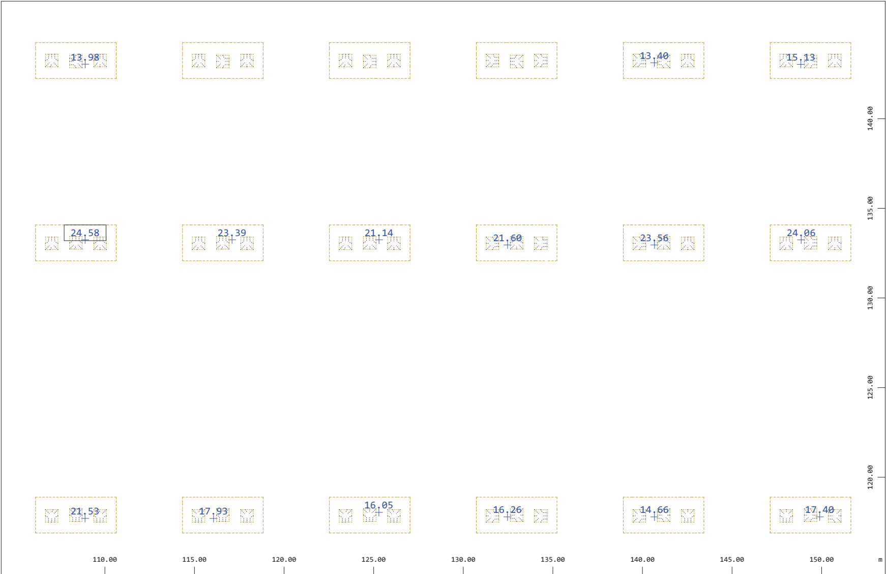
Sector of system Group 15 Quadrilateral Elements , Shear reinforcement in cm2/m2, Design Case 1 , Values greater than 13.26 (Max=24.58)
